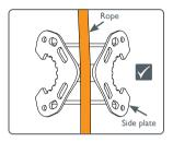
The positioning of the rope on the Edge Guard may be affected by rope deviations below the Edge Guard and changes in work position while carrying out the work task; ensure that the Edge Guard is positioned accordingly before beginning work. Beware, the greater the distance between the Edge Guard and the anchor point, the greater the potential for lateral movement of the rope.
