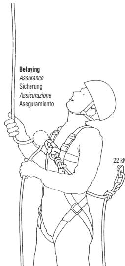
This product is designed and manufactured to be used in conjunction with a dynamic UIAA rope. If used together with static equipment alone (low-stretch rope, tape slings...) and if there is a risk of a fall, it is essential to introduce a shock-absorber into the safety chain to lower the potential shock load.
